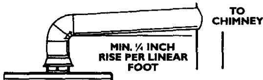
VENT PIPE INSTALLATION
