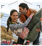
Framing marks indicate the camera focus area.
