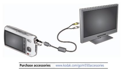
NOTE: Ensure that the Video Out setting (NTSC or PAL) is correct (see page 36). The slide show stops if you connect or disconnect the cable while the slide show is running. (Image quality on a television screen may not be as good as on a computer monitor or when printed.)
