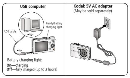
NOTE: Rechargeable batteries have a limited number of charging cycles. Battery life and number of charge cycles vary by use and settings.
