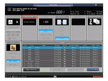
**5** Press [▶] on the right side of [Screen Pattern] to display the desired screen.
