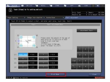
**13** When the [PRINT MODE] screen is displayed, press **Start** on the **control panel**. A test chart is printed. Output about 3 sheets.
