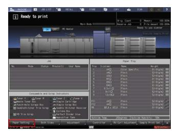
11 Select the tray in which the paper to be adjusted has been loaded, then press [Change Set].
