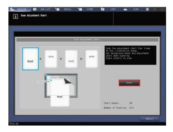
When scanning is properly completed, the counter of [Number of Scanning] on the [Scan Adjustment Chart] screen is added by one, and the blue frame displayed in the illustration on the screen shifts to the next one on the right side. If you move the adjustment chart before the blue frame shifts to the next, the measurement may not be performed properly.
