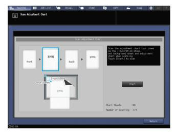
Third time: Set the back side of the adjustment chart face up (turned away from the **original glass**), with its top edge positioned to the back side.
