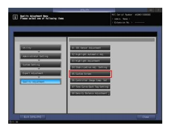
Press the screen to be assigned to each screen type: [Screen1], [Screen2], and [Stochastic]. After setting, press [OK].
