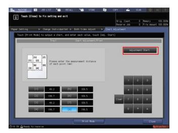
14 Output the front side adjustment chart again, then check the lengths at points [2], [4], [6], and [8] on the second and third output charts.
