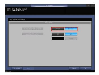
When **Intelligent Quality Optimizer IQ-501** is mounted on the machine, this option is always set to [Precise].
