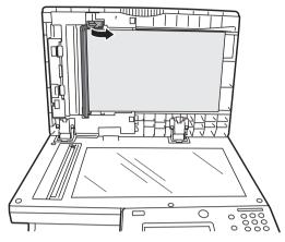
${f 8}$  Use a soft cloth moistened with water and well-wrung to clean the face of the rollers.
