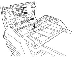
Rotate the rollers by hand to clean the entire roller surface.
