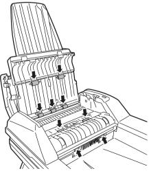
Rotate the rollers by hand to clean the entire roller surface.
