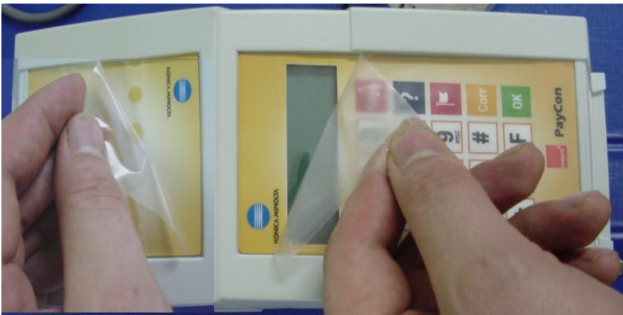
9. Remove the transport foils to finish the installation
