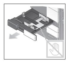
Slide the Lateral Guide to fit the size of the paper to be loaded.
