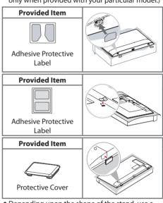
• Depending upon the shape of the stand, use a flat tool to remove the stand cover as illustrated below. (e.g., a flat screwdriver)
