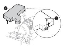
Remove the cover and pull out the tube <sup>(a)</sup>.Disconnect all wire harnesses <sup>(a)</sup>. Unscrew the ground wire <sup>(b)</sup>.
