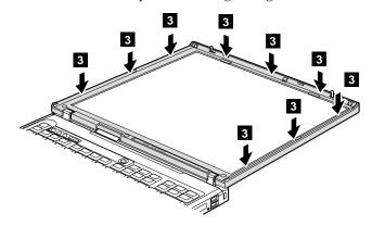
3. Attach the LCD rear cover from the top end.
