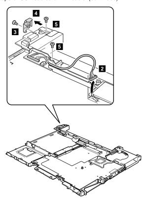
In step 4, remove the security hole bracket in the direction of the arrow.
