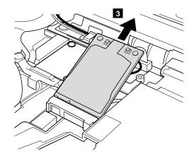
Table 20. Installation of the PCI Express Mini Card for wireless LAN
