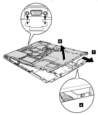
Table 30. Installation of the PC Card slot bezel
