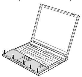
4. Close the LCD cover, and turn the computer over. Then fasten the four screws to secure the palm rest.
