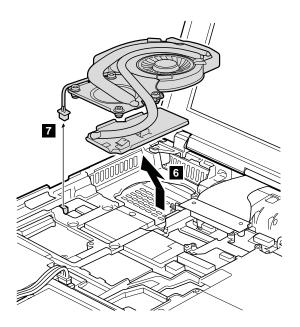
Table 26. Installation of the fan assembly
