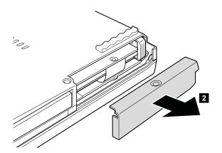
Table 13. Removal steps of HDD cover, HDD, and HDD rubber rails (continued)
