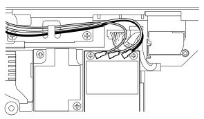
• After you secure the card, make sure that the antenna cables are routed as shown in the each figure.
