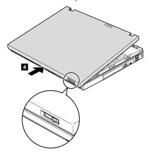
4. Attach the latches of the LCD rear cover firmly.
