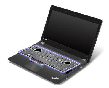
3. Slide the keyboard in the direction shown by the arrows,until the keyboard is secured in place.
