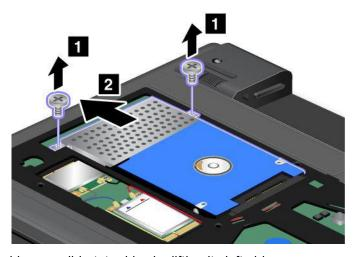
6. Remove the hard disk drive or solid-state drive by lifting its left side.
