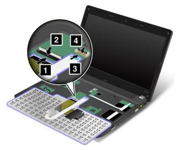
2. Insert the keyboard. Make sure that the rear edge of the keyboard is under the frame.
