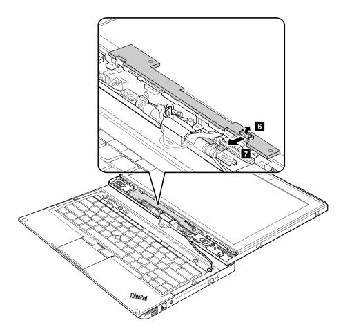
When installing: Ensure that the connector is attached firmly.
