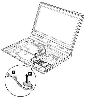
When installing: Ensure that the battery connector is attached firmly.
