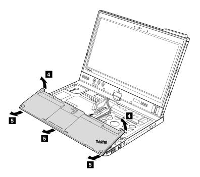
When installing: Press the front edge of the palm rest to fit it into place 1. Then, press the rear edge of the palm rest until it clicks into place 2.
