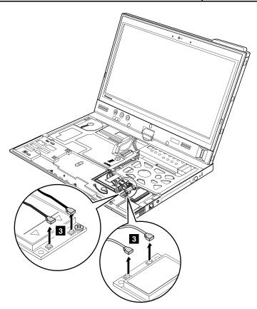
In step 4, release the wireless antenna cables from the cable guides.
