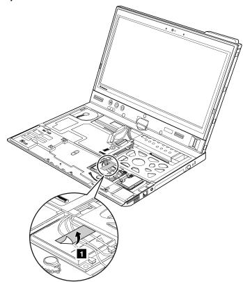
Unplug the connectors by using the antenna RF connector removal tool or pick the connectors with your fingers and gently unplug them in the direction of the arrow 2.
