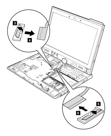
When installing: Ensure that the connectors are attached firmly to the system board.
