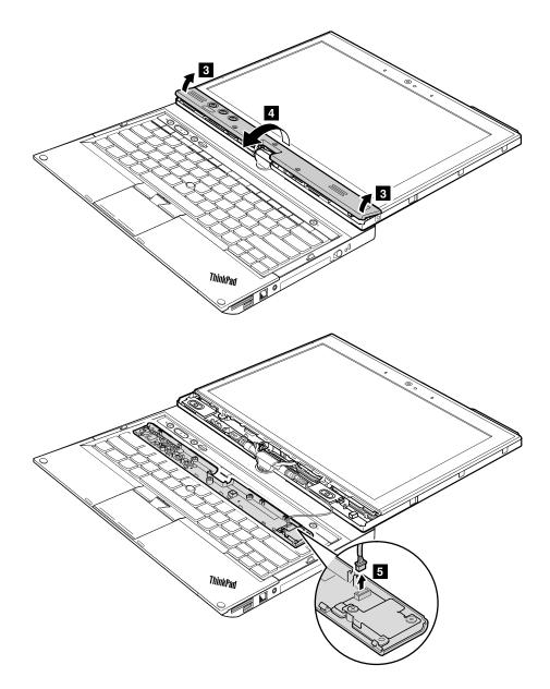
When installing: Ensure that the connector is attached firmly.
