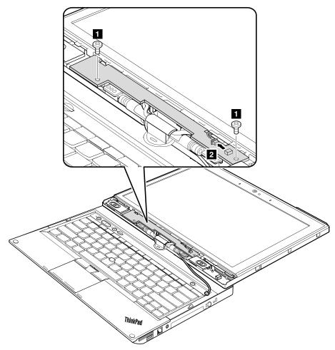
When installing: Ensure that the connector is attached firmly.
