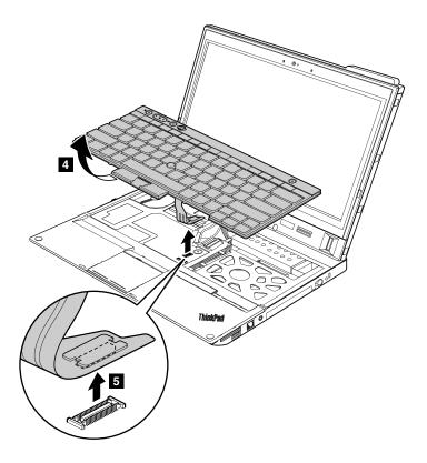
When installing: Ensure that the keyboard connector is attached firmly.
