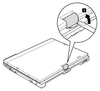
Open the LCD unit, and then remove the hinge cap.
