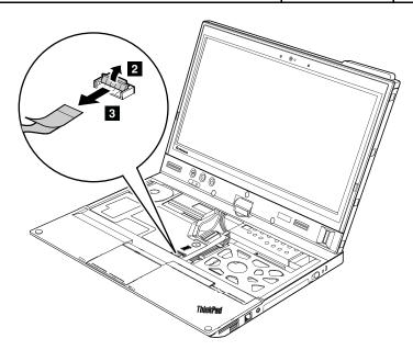
When installing: Ensure that the connector is firmly attached to the system board.
