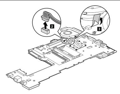
When installing: Ensure that the connector is attached firmly to the system board.
