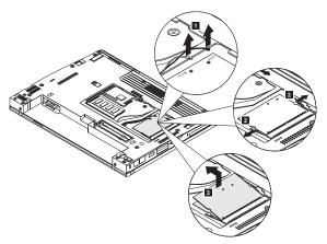
Pull over the levers to detach DIMM.
