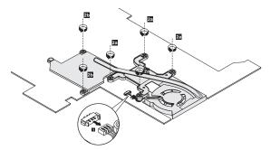
Remove Fan cable then release four screws to remove Fansink for the models with LV processor.
