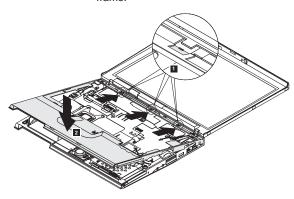
Note: After installing upper case, arrange antenna as 1. If BMDC-3 is used, arrange antenna as 2.
