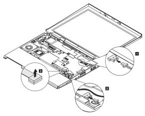
Gently push the upper case backward, as shown in step 1. And lift it up slightly, as shown in step 2. Then release the latches, as shown in step 3 and step 4, carefully to remove the upper case.
