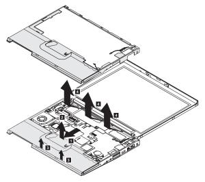
When installing: Make sure that the upper case edges, shown in the step 1, are under the frame.
