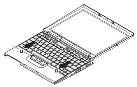
Secure the keyboard by tightening the screws from the bottom side of the computer.
