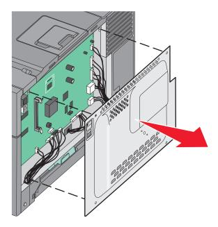
**4** Locate the appropriate connector on the system board.
