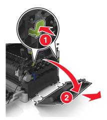
Press the green levers on each side of the waste toner bottle, and then remove the waste toner bottle.
