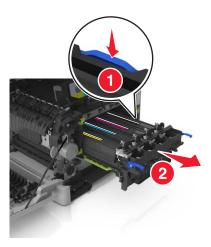
**8** Remove the used developer unit.
