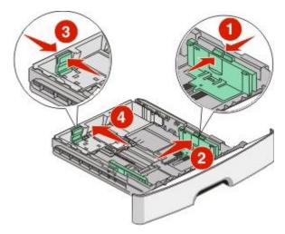
If you plan to load a non-standard (Universal) paper size that does not have a defined stop in the bottom of the tray, wait to adjust the length guide until paper is loaded. Adjust the length guide to lightly touch the back of the stack of paper. Adjust the length guide properly to alleviate repeated jams and paper feeding problems.
