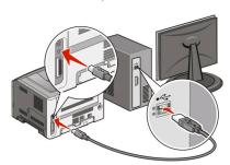
**Note:** After the printer is configured, the software will instruct you to disconnect the temporary USB cable so you can print wirelessly.
