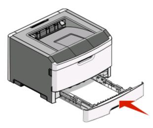
**8** If a different type of paper was loaded than the type previously loaded in the tray, change the Paper Type setting for the tray from the printer control panel. For more information, see "Setting the Paper Size and Paper Type" on page 38.
