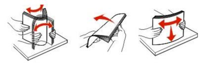
Turn the stack of paper over, if possible, when you reload it into the tray or feeder.
