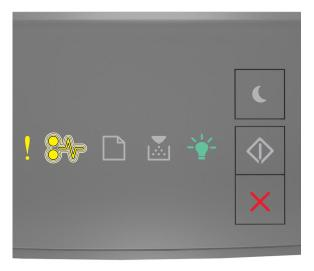
If the supplemental light sequence matches the light sequence in the preceding illustration, then replace the toner cartridge. For more information, see the instruction sheet that came with the supply or see the "Replacing supplies" section of the *User's Guide*.
