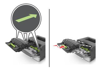
7 Insert the toner cartridge into the printer by aligning the side rails of the cartridge with the arrows on the side rails inside the printer.
