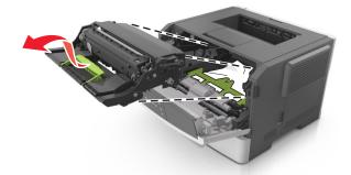
**Warning—Potential Damage:** Do not expose the imaging unit to direct light for more than 10 minutes. Extended exposure to light may cause print quality problems.
