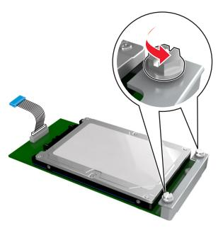
**b** Align the screws on the printer hard disk to the slots on the controller board bracket, and then slide the printer hard disk onto the brackets.
