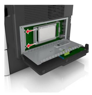
**c** Tighten the two screws.
