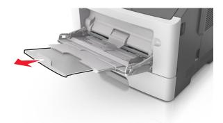
2 Squeeze the tab on the left width guide, and then move the guides for the paper you are loading.
