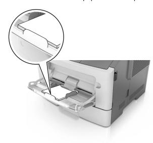
• Load letterhead faceup with the top edge entering the printer first. For two-sided (duplex) printing, load letterhead facedown with the bottom edge entering the printer first.
