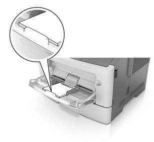
• Load letterhead faceup with the top edge entering the printer first. For two-sided (duplex) printing, load letterhead facedown with the bottom edge entering the printer first.
