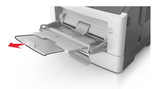
2 Squeeze the tab on the left width guide, and then move the guides for the paper you are loading.
