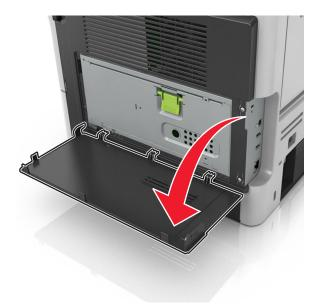
**2** Open the controller board shield using the green handle.
