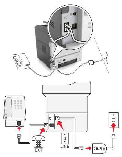
Digital subscriber line (DSL) splits your regular telephone line into two channels: voice and Internet. Telephone and fax signals travel through the voice channel, and Internet signals pass through the other channel.
