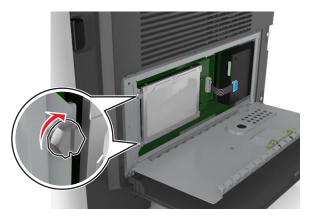
4 Close the controller board shield, and then close the controller board access door.
