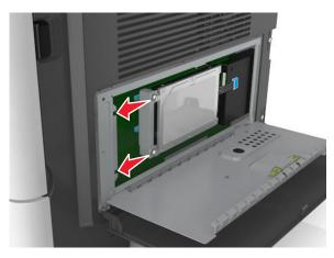
**d** Tighten the two screws.
