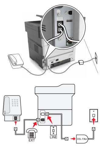
Digital subscriber line (DSL) splits your regular telephone line into two channels: voice and Internet. Telephone and fax signals travel through the voice channel, and Internet signals pass through the other channel.
