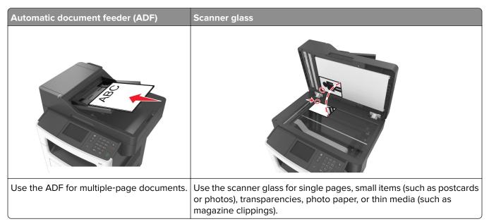
The scanner lets you scan documents directly to a computer or a flash drive. The computer does not have to be directly connected to the printer for you to receive Scan to PC images. You can scan the document back to the computer over the network by creating a scan profile on the computer and then downloading the profile to the printer.
