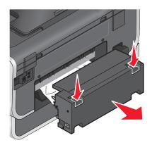
**CAUTION—POTENTIAL INJURY:** The area behind the duplex cover has protruding ribs as part of the paper path. To avoid injury, use caution when accessing this area for clearing a paper jam.
