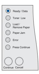
The operator panel has six lights and two buttons. Lights that are on, off, or blinking indicate different printer conditions. For full information on the operator panel, refer to the *Publications* CD.
