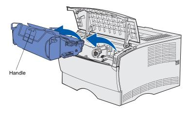
2 Grasp the print cartridge by the handle. Lift the cartridge out of the printer.
