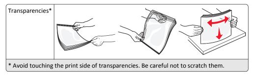
**5** Load the paper or specialty media. Slide the stack gently into the multipurpose feeder until it comes to a stop.
