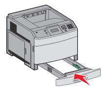
**8** If a different type of paper was loaded than the type previously loaded in the tray, then change the Paper Type setting for the tray from the printer control panel.
