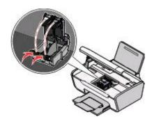
7 Remove the tape from the black cartridge, insert the cartridge in the left carrier, and then close the black cartridge carrier lid.
