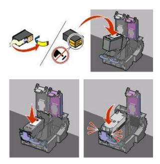
**8** Remove the tape from the color cartridge, insert the cartridge in the right carrier, and then close the color cartridge carrier lid.
