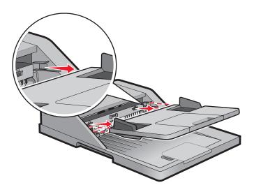
**2** Remove the jammed paper by pulling the lower edge of the sheet exiting the ADF.
