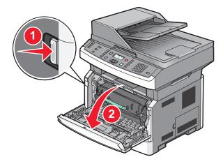
**2** Press the button on the base of the photoconductor kit, and then pull the toner cartridge out using the handle.
