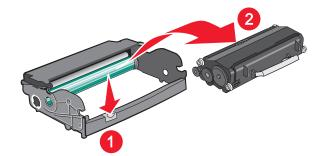
**5** Unpack the new photoconductor kit. Be careful not to touch the photoconductor drum.
