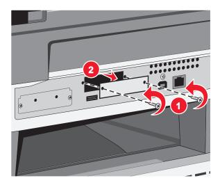
4 Insert the fax card, and then tighten the two screws to secure the fax card mounting bracket.
