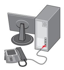
**6** Connect an additional telephone cord from the computer modem LINE port  $\stackrel{[a]}{=}$  to the printer EXT port  $\stackrel{[a]}{=}$ .
