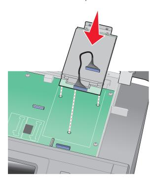
**b** Attach the two provided screws to secure the printer hard disk mounting bracket.
