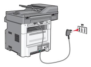
4 If you would like to use the same line for both fax and telephone communication, then connect a second telephone line (not provided) between the telephone and the F slot of an active analog telephone wall jack.
