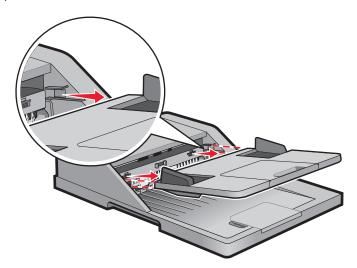
**2** Pull out the jammed paper by pulling the sheet on the bottom.
