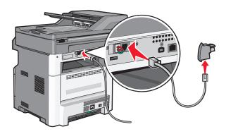
**3** Connect the adapter into the N slot of an active analog telephone wall jack.
