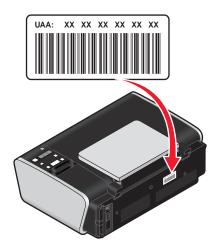
**Note:** A list of MAC addresses can be set on an access point (router) so that only devices with matching MAC addresses are allowed to operate on the network. This is called MAC filtering. If MAC filtering is enabled in your access point (router) and you want to add a printer to your network, the MAC address of the printer must be included in the MAC filter list.
