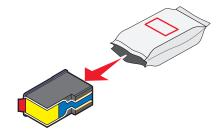
**11** If a storage unit is included, remove the color cartridge from the storage unit.
