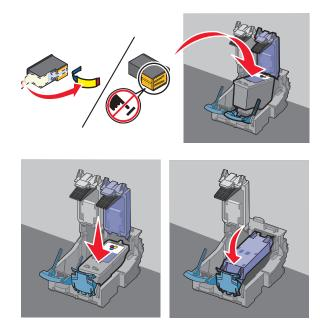
**13** If a black print cartridge is included in the box contents, open the black cartridge foil, and then remove the cartridge from the pack.
