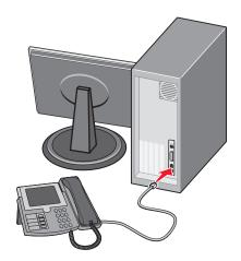
**6** Connect an additional telephone cord from the computer modem LINE port = to the printer EXT port =.
