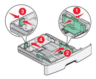
For long paper like A4 or legal, squeeze and slide the length guide backwards to accommodate the length of paper you are loading.
