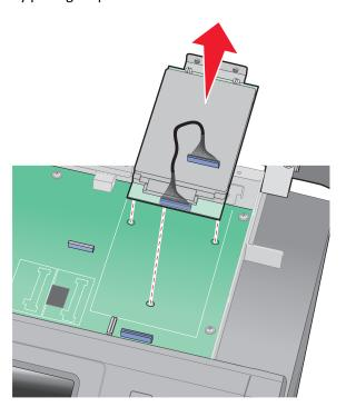
**d** Remove the thumbscrews that attach the printer hard disk mounting bracket to the printer hard disk, and then remove the bracket. Set the printer hard disk aside.
