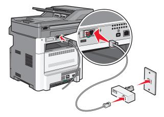
**3** Connect the answering machine or telephone to the adapter.
