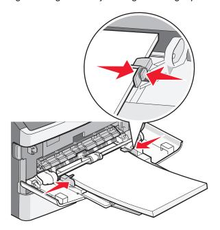
5 Slide the paper gently into the multipurpose feeder until it comes to a stop. Paper should lie flat in the multipurpose feeder. Make sure the paper fits loosely in the multipurpose feeder and is not bent or wrinkled.
