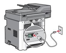
**3** Remove the plug from the printer EXT port :
