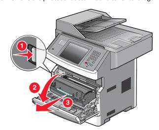
2 Lift the flap at the front of the printer, and then remove any jams.
