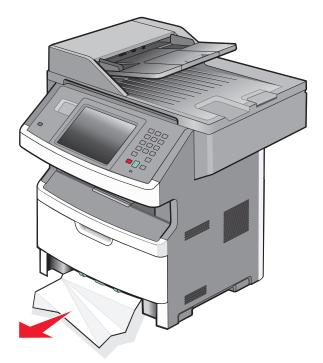
If you do not see the jam, open the front door, and then remove the photoconductor kit and toner cartridge.
