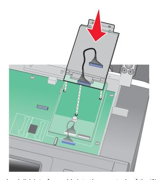
**c** Insert the plug of the printer hard disk interface cable into the receptacle of the ISP.
