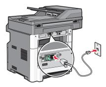
**4** Remove the protective plug from the printer EXT port :
