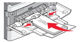
**Warning—Potential Damage:** Never use envelopes with stamps, clasps, snaps, windows, coated linings, or self-stick adhesives. These envelopes may severely damage the printer.
