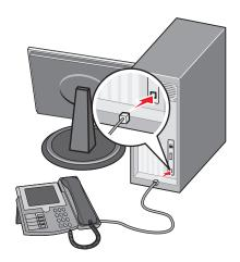
**5** Connect a third telephone cord from the computer modem to the bottom EXT port  $\widehat{}_{||}$  of the printer.
