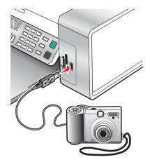
The message PictBridge camera detected. Press  $\checkmark$  to change settings. appears on the display.
