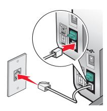
**3** Remove the protective plug from the EXT port  $\stackrel{\frown}{=}$  of the printer.
