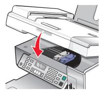
The control panel display will prompt you to load paper and press **(**) to print an alignment page.
