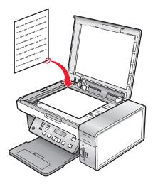
Close the top cover to avoid dark edges on the scanned image.
