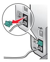
**4** Connect the other telephone cord to a telephone, and then plug it into the EXT port  $\stackrel{\frown}{=}$  of the printer.
