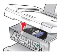
**3** Press down on the cartridge carrier latch to raise the cartridge carrier lid.
