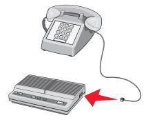
**5** Connect a third telephone cord from the answering machine to the EXT port of the printer.
