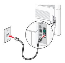
**3** Remove the protective plug from the EXT port  $\widehat{}_{||}$  of the printer.
