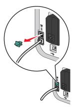
**4** Connect the other telephone cord to a telephone, and then plug it into the EXT port of the printer.
