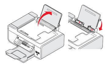
**8** Load paper, and then pull up the paper adjustment lever to adjust the paper guides. The paper guides should rest against the edges of the paper.
