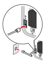
**3** Remove the protective plug from the EXT port of the printer.
