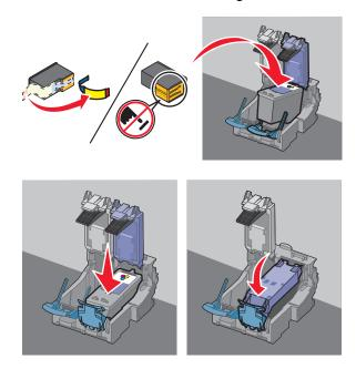
**Warning—Potential Damage:** Do *not* touch the gold contact area on the back or the metal nozzles on the bottom of the cartridge.
