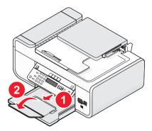
7 Raise the paper support, and then press down on the paper adjustment lever to extend the paper guides.
