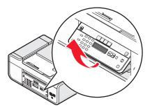
**4** If a stick-on overlay for your language needs to be installed, peel off the covering from the back of the overlays to expose the adhesive.
