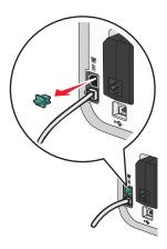
**4** Connect a second telephone cord from the computer modem to the EXT port of the printer.
