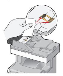
**9** Pull the flap up as shown, and then wipe the sensor behind it.
