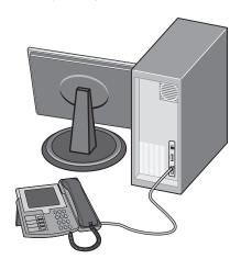
**5** Connect an additional telephone cord (not provided) from the computer modem to the printer EXT port  $\widehat{\mathbb{H}}$ .
