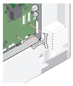
7 Install the ISP on the plastic tee. Angle the ISP over the plastic tee, and then slant it toward the plastic tee so that any overhanging connectors will pass through the ISP opening in the system board cage.
