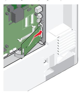
Lower the ISP toward the plastic tee until the ISP is seated between the guides of the plastic tee.
