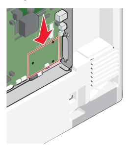
Note: If an optional ISP is currently installed, then the printer hard disk must be installed onto the ISP.
