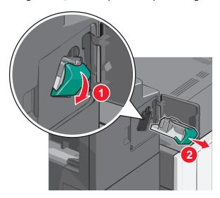
**3** Use the metal tab to lift the staple guard, and then remove any jammed or loose staples.
