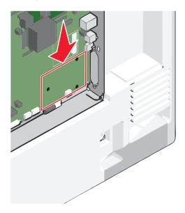
Remove the printer hard disk.
