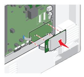
**d** Insert the plug of the printer hard disk interface cable into the receptacle of the ISP.
