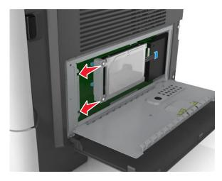
**d** Tighten the two screws.
