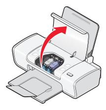
Press down on the cartridge carrier lever to raise the cartridge carrier lid.
