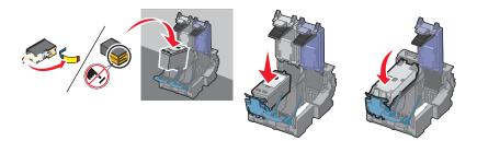
**Warning—Potential Damage:** Do *not* touch the gold contact area on the back or the metal nozzles on the bottom of the cartridge.
