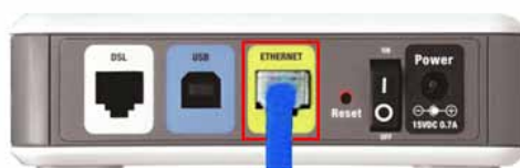
Back view of DSL modem
