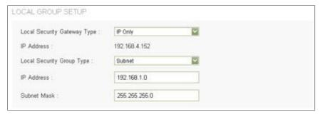
• Local/Remote Security Gateway Type: This Local Security Gateway Type must be identical to the Remote Security Gateway Type of the remote peer.
