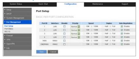
The default port settings will be sufficient for most small businesses, but you can still use the *Port Management > Port Setup* page to customize these settings. You can disable a port or customize its priority, speed, duplex mode, and autonegotiation settings. You can also enable port-based VLANs to control traffic between devices on your network.
