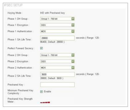
Enter the settings for IKE with preshared key mode. Be sure to enter the same settings when configuring the other end router for this tunnel.
