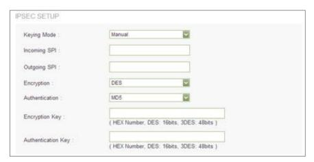
Enter the settings for manual mode. Be sure to enter the same settings when configuring the other end router for this tunnel.
