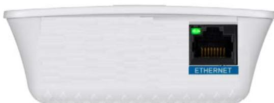
**Ethernet** (blue) Connect wired devices to your wireless network with Ethernet (network) cables. The green light turns on when an Ethernet device is connected and active on this port. The light blinks when the extender is sending or receiving data over the Ethernet port.
