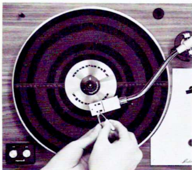
Figure 4. Stylus Overhang Adjustment
