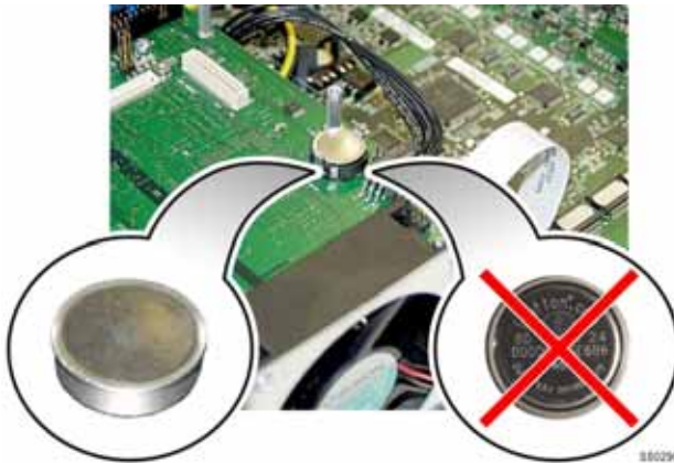
Figure 40: Installing the System i-Button
