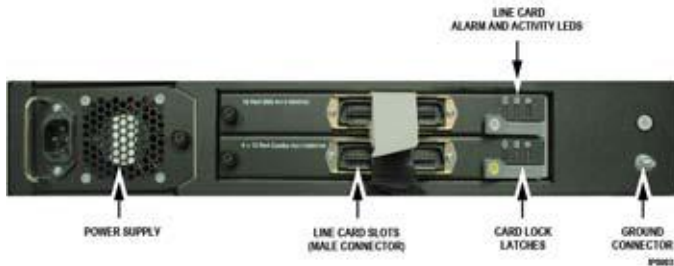
Figure 118: ASU II – Back Panel with a Line Card
