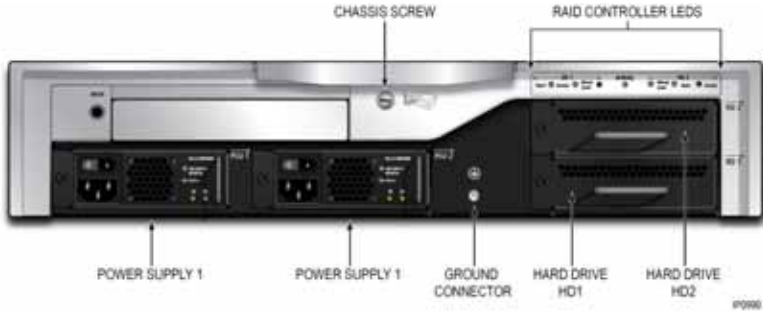
Figure 97: Mx Server – Back panel
