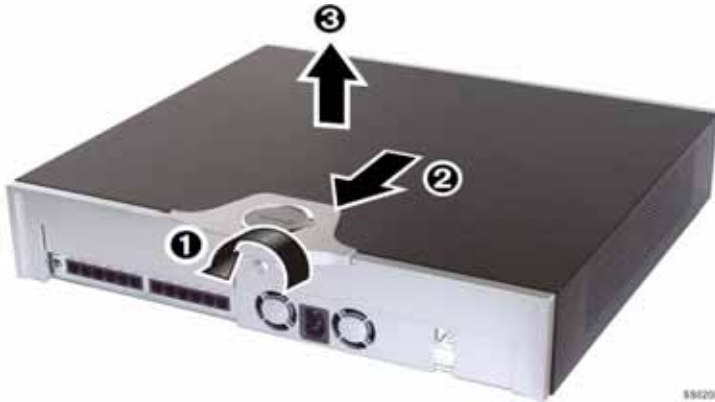
Figure 11: CX/CXi, CX II/CXi II - Removing the cover
