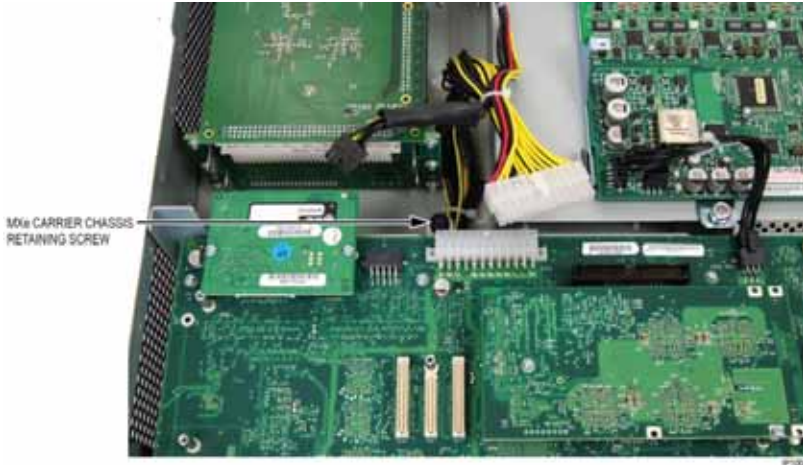
Figure 34: Carrier Chassis Retaining Screw
