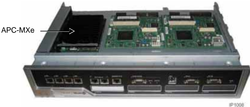
Figure 51: APC-MXe on MXe Carrier Board
