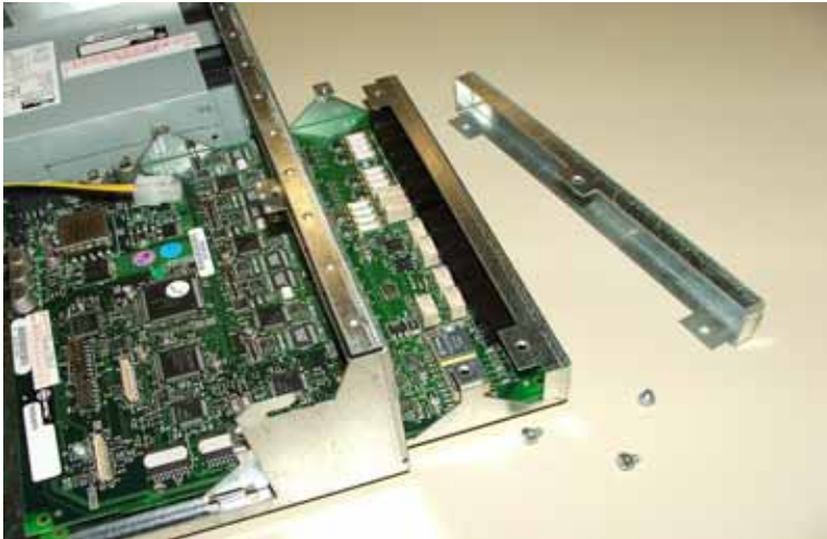
Figure 42: CX/CXi, Insert the Analog Main Board
