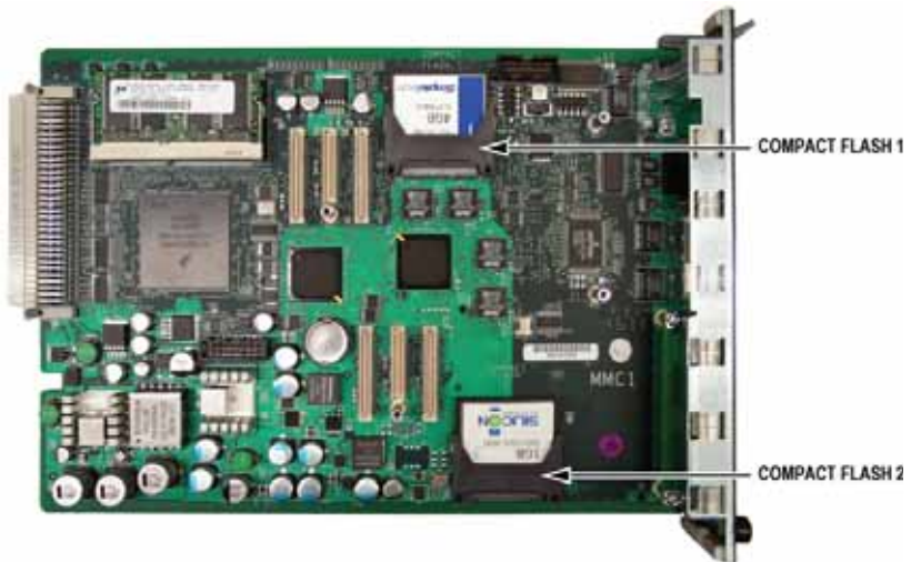
Figure 85: AX Flash 1 and Flash 2 Locations
