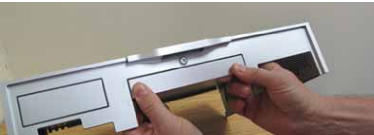
Figure 46: Remove Blanking Panel
