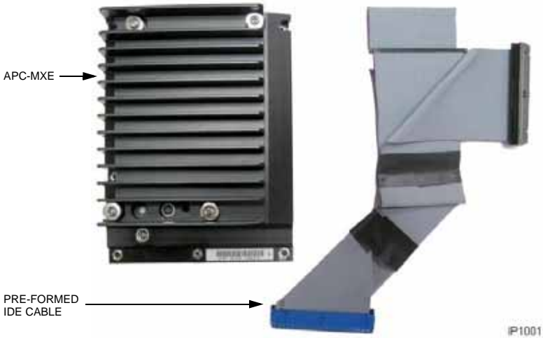
Figure 31: APC-MXe and Pre-formed IDE Cable
