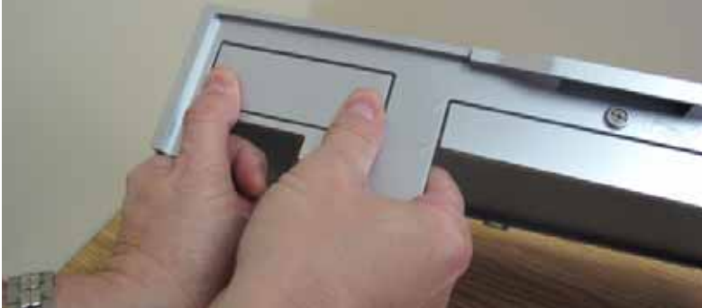
Figure 66: Remove Blanking Plate
