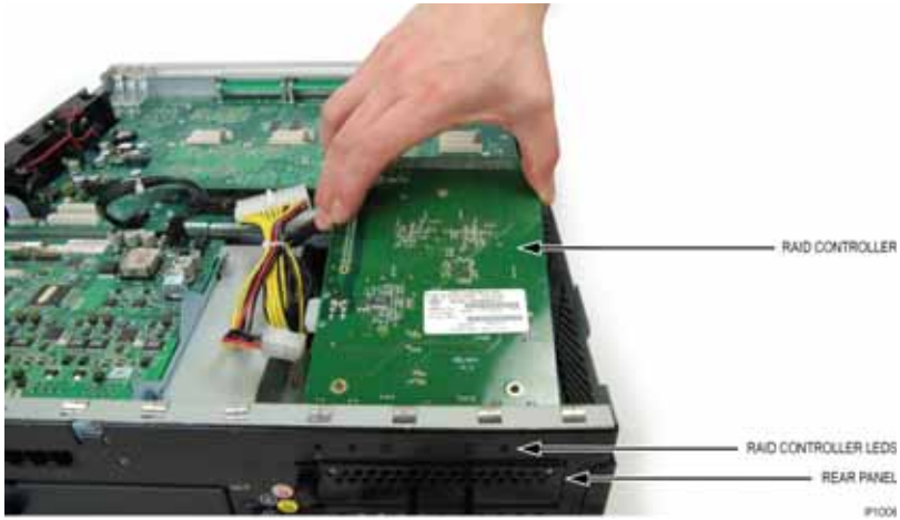
Figure 79: Position the RAID Controller Board
