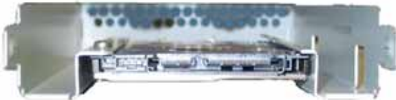
Figure 75: Hard Drive / SSD Installed in Drive Carrier
