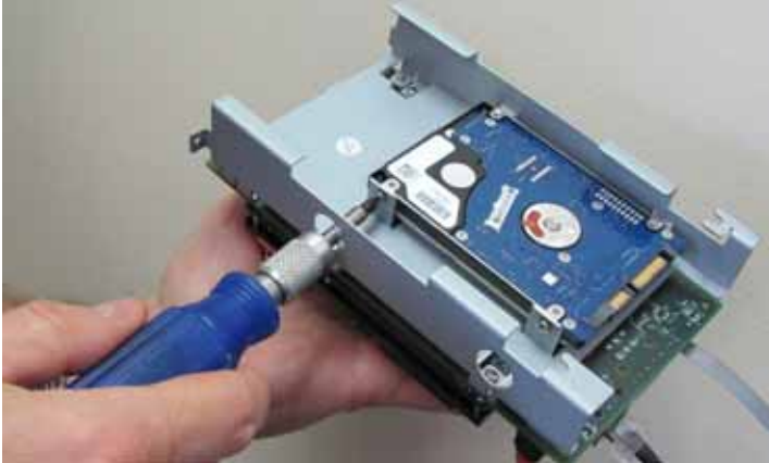
Figure 67: APC-CX(i) II Hard Disk Drive Removal
