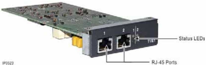
Figure 150: Dual T1/E1 Framer Module
