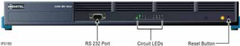
Figure 155: BRI NSU LEDs
