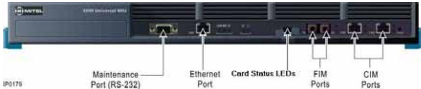
Figure 154: Universal and R2 NSU LEDs
