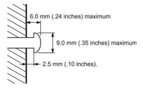
Note: Example above for mounting SBV5220 on a wood surface.
