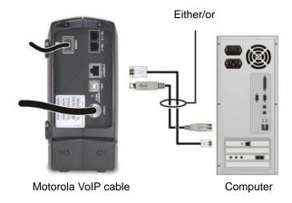
**USB:** Be sure the SBV5220 VoIP Cable Modem CD-ROM is inserted in your CD-ROM drive. Perform the appropriate procedure for Setting Up a USB Driver for your Windows version. Connect the USB cable to the USB port on the Motorola VoIP cable modem. Connect the other end to the USB port on your PC.
