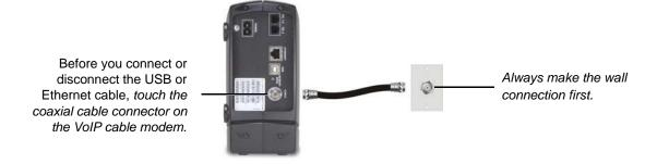
To prevent overheating the VoIP cable modem, do not block the ventilation holes.
