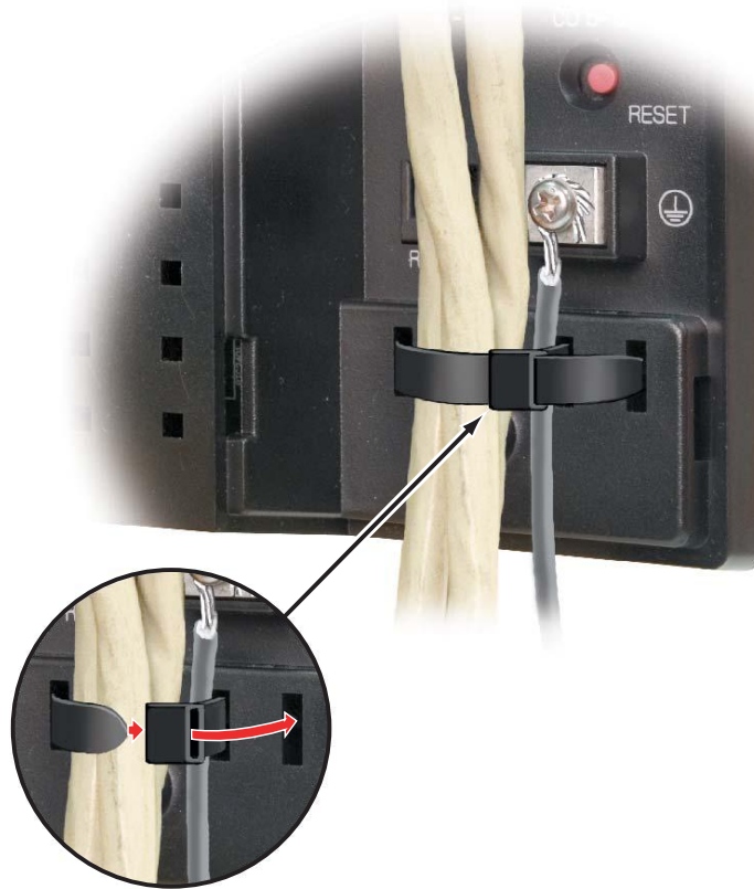
Figure 11: Securing the Cables
