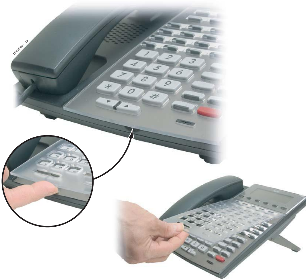
Figure 21: Removing the Telephone Faceplate
