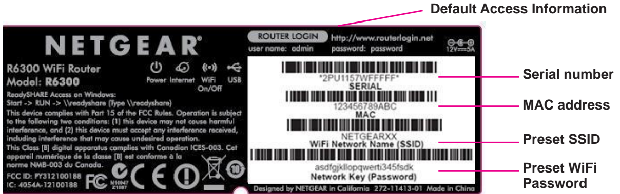
Figure 4. The label shows unique information about your router
