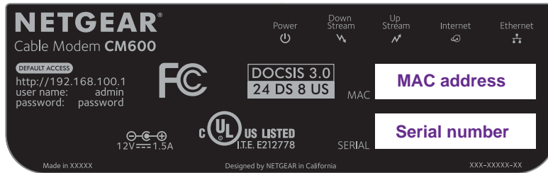
Figure 6. Find the serial number and the MAC address on the product label
