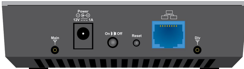
Figure 4. Modem components on the back panel
