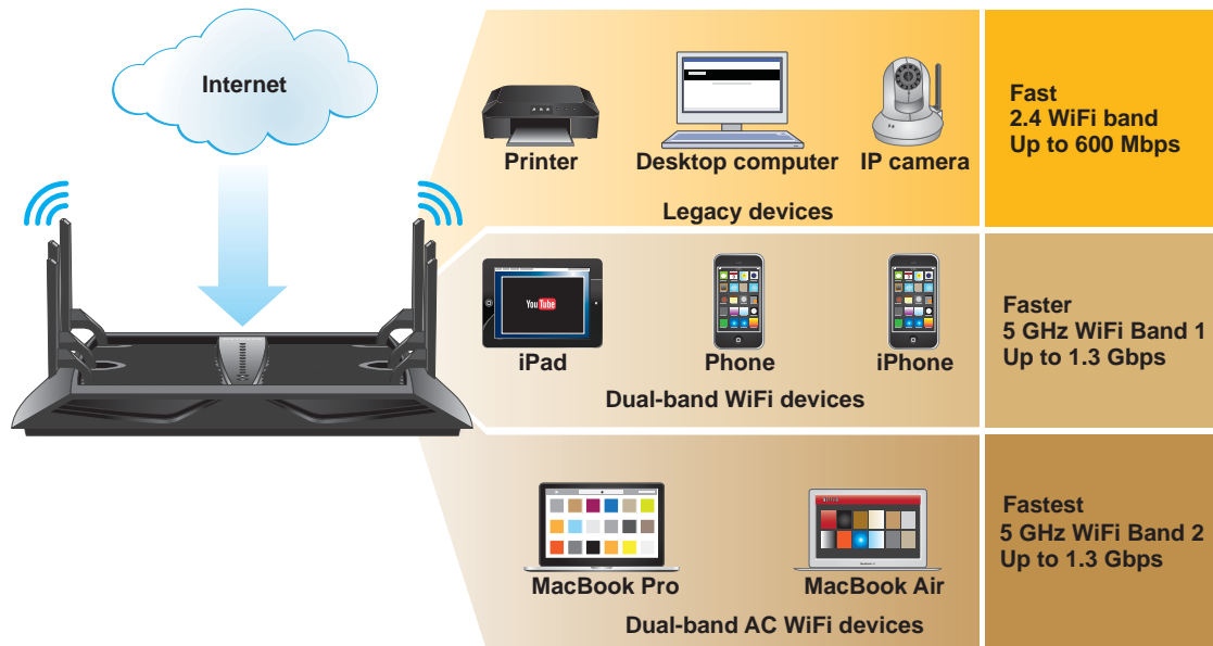
Figure 9. Load balancing in a tri-band WiFi network
