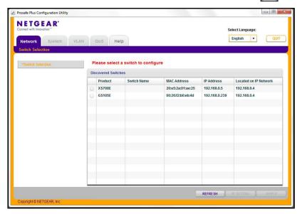
The Switch Selection page displays a list of Web Managed (Plus) switches that the utility discovers on the local network.
