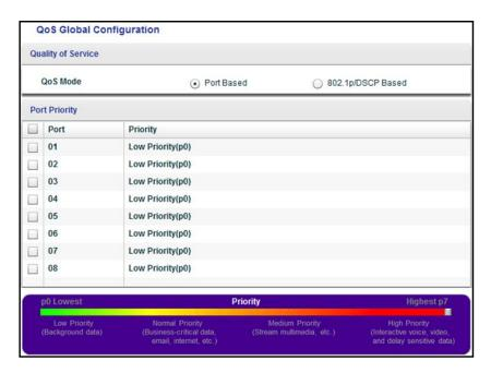
The previous figure is an example. Your switch might provide more or less ports. The **802.1p/DSCP-based** radio button is not supported on all models and therefore might not show on the page.
